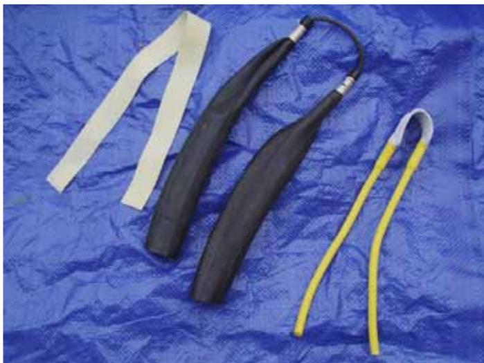
Here are three types of elastics, surgical webbing, a bike inner tube with paracord string attachment and a commercial sling shot band.
